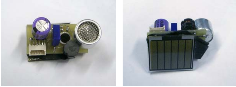
Fig. 6. Light-powered beacon, top view and bottom view. The solar panel measures 23 by 20 mm, the unit is mounted by means of Blue-tac.
