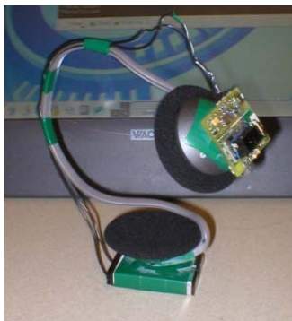
Fig. 1. The FreeDiger device is equipped with a dual axis accelerometer, an infrared proximity sensor, and a Bluetooth radio for wireless communication. The entire device is worn like a pair of headphones with the sensors positioned over one of the ears.
