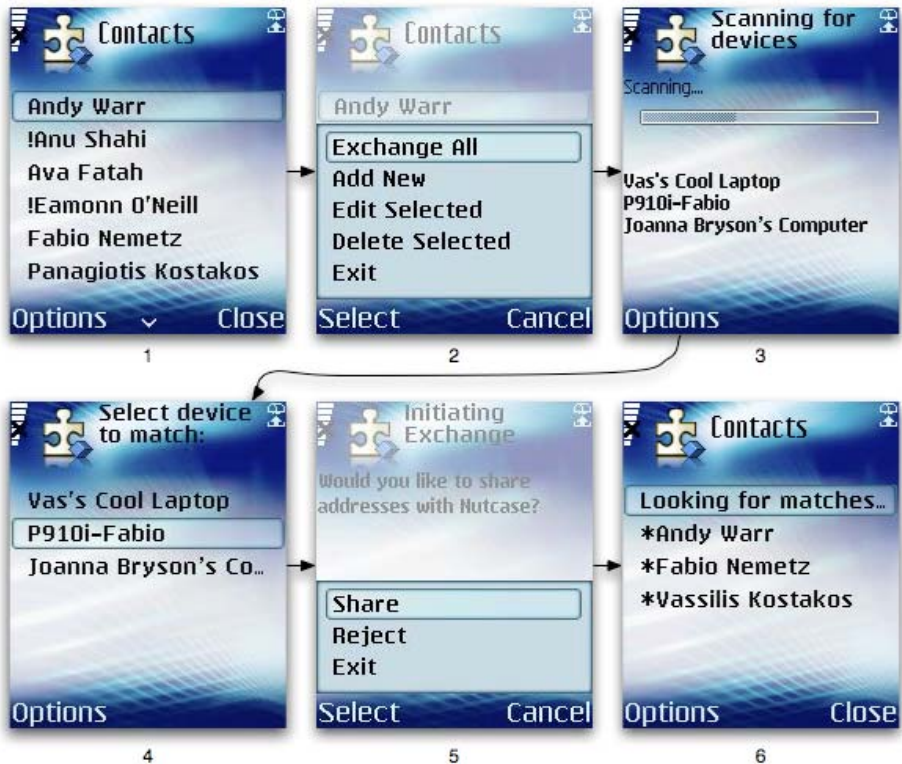
Fig. 3. Using Bluetooth, a user needs to activate the exchange mechanism (photos 1 to 4). The other user is alerted to the request for exchange (photo 5). If the user agrees, the phones carry out a two-way exchange of digests. Upon successful completion of the exchange, the phones present the common entries (photo 6).
