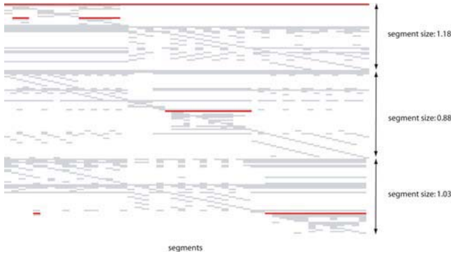
Fig. 5. Result of applying the adapted algorithm to the signal shown in Figure 4. Three different segment sizes between 0.88 and 1.18 seconds were used.
